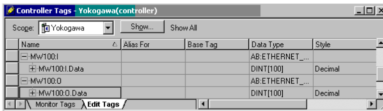
MW100 Channels within RSLogix 5000 Controller Tags Screen.
